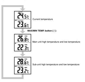
To clear the high temperature and low temperature data memory, press the CLEAR button (®).
